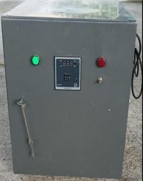
This is a machine ,it is used to generates foam from foaming agent liquid , after making of foam ,it is use to make CLC block and Light Mix Concrete ,which is also called light weight foam concrete. All the specifications are mentioned below.
